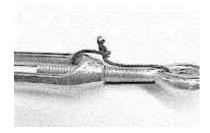
The main frames must be aligned with the frame x-bracing in the back. Measure the distance between the frame cross-brace below the chrome wheel and the side of the right channel. This space should be 3 1/2". Adjust the rear turnbuckles to make this space 3 1/2". To increase the gap, loosen the right turnbuckle and tighten the left. To reduce it, loosen left and tighten right.
