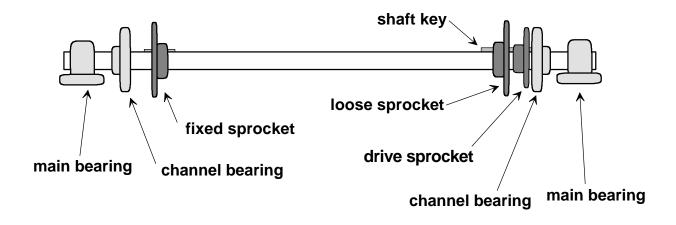
Note that the *fixed sprocket* goes to the left. The *loose sprocket* remains free to slide back and forth so that it can self-align when the panels are in place. The smaller *drive-sprocket* will be fastened down with setscrews when the drive chain is installed.
