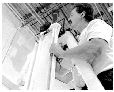
The *pulley-bar* is a large part with "Treadwall" printed on it in big letters. It goes between the two channels at the top of the machine.
