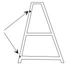
The *horizontal braces* are long rectangular tubing with L-shaped fittings welded to each end.
